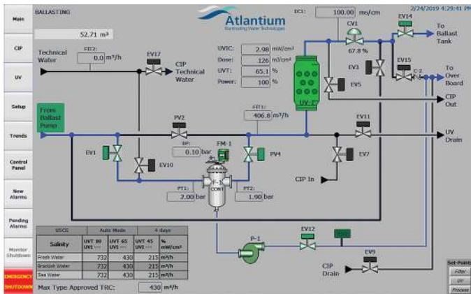
Operators select the Authority (IMO or USCG) for intended location of de-ballasting and the holding time. Then the ballasting or de-ballasting process is selected. The One-Pass™ ballasting mode can also be selected at this time if desired.
