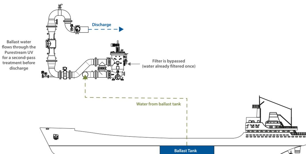
Purestream system is validated to operate at **minimum retention times** ( $\leq 24$  hours) following treatment under difficult water conditions with UV transmittance as low as **40% UVT**.
