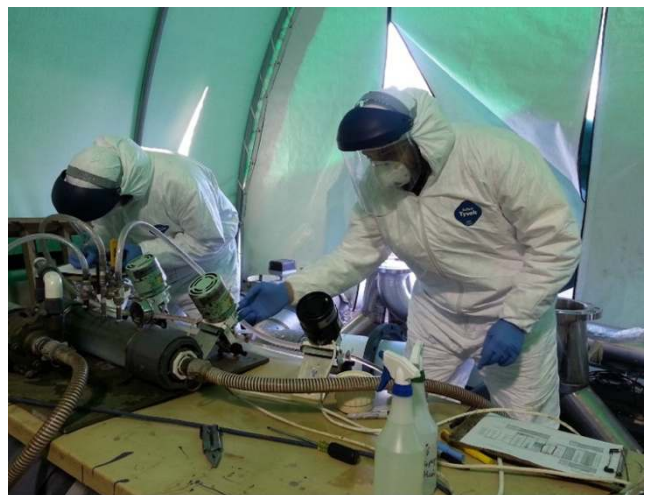
Figure 1: Hydro-Optic™ (HOD) UV validated to U.S. EPA guidelines for 4-log virus inactivation using real adenovirus, not a surrogate.
