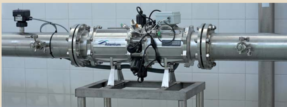
Fig. 4 Tested RZ-163 system model including sensor placement and ultrasound cleaning
