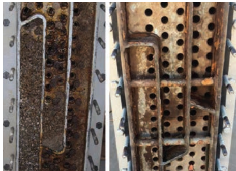
1. A Parker Dam heat exchanger that was pulled for maintenance before the Hydro-Optic ultraviolet (HOD UV) treatment implementation (left), and the same unit, exposed for the same time and similar conditions, after treatment with HOD UV (right). Courtesy: Parker Dam staff/Bureau of Reclamation
