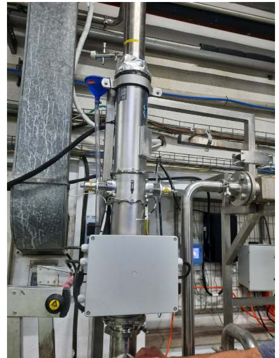
Atlantium's Hydro-Optic™ (HOD) UV system delivers unprecedented microbial inactivation to a pasteurized equivalent without the use of heat.
