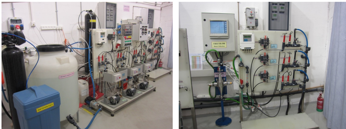
Figure 2-3 Bench-scale evaluations of HOD UV technology for dechlorination
