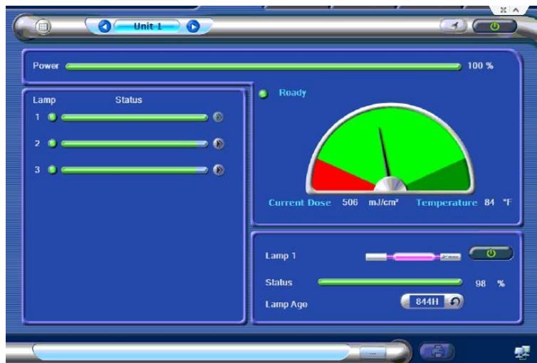
Figure 3-4 HOD UV remote access display
