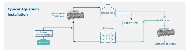
Atlantium's HOD™ system can be used for Flow-through, Recirculation and Effluent applications in any location
