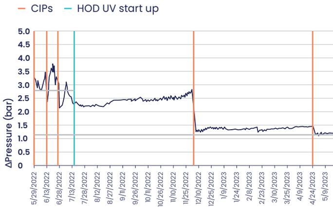
Transmembrane pressure differential ( $\Delta P$ ) achieved the lowest post-CIP  $\Delta P$  (> 20 psi), which was never seen before. This means the changes in biofilm structure (less EPS) make CIP more effective, cleaning membranes more deeply, and even better, after the second CIP.
