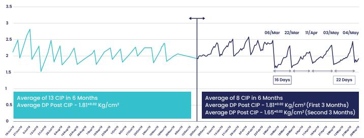
RO differential pressure prior to and post HOD UV technology installation
