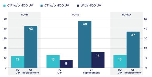
Performance data comparison for RO train with HOD UV protection (RO Train 12) and the same RO train six months before HOD UV installation (RO Train 12A), and for an RO train without HOD UV protection (RO Train 11).
