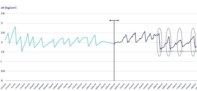
CIP is more efficient – 0.75 kg/cm<sup>2</sup> vs. 0.59 kg/cm<sup>2</sup> before HOD UV installation
