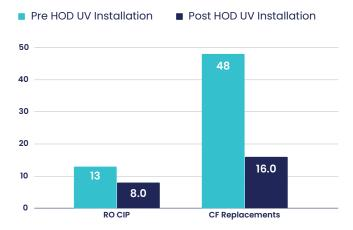
RO CIP frequency and CF replacement frequency, six months before and after HOD UV installation.
