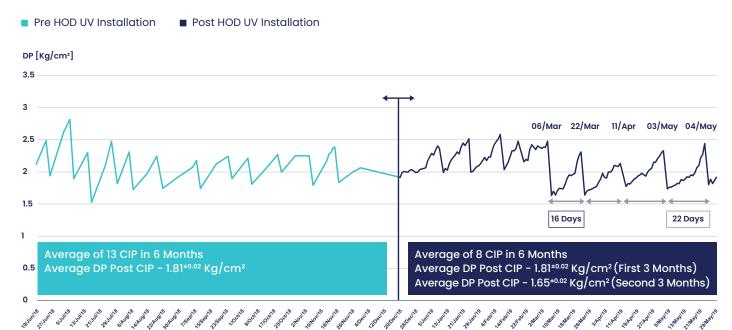
RO differential pressure prior to and post HOD UV technology installation
