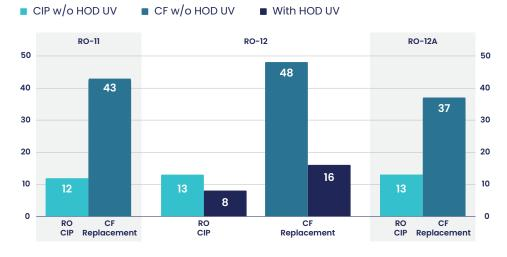
Performance data comparison for RO train with HOD UV protection (RO Train 12) and the same RO train six months before HOD UV installation (RO Train 12A), and for an RO train without HOD UV protection (RO Train 11).
