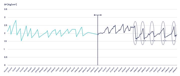
CIP is more efficient – 0.75 kg/cm² vs. 0.59 kg/cm² before HOD UV installation
